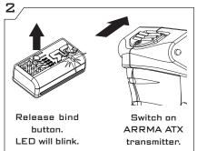
To start binding the ARRMA transmitter and receiver, ensure that both units are switched off, within 30cm/12" of each other and clear of possible sources of interference.
