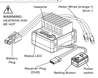
The MEGA waterproof brushed ESC (electronic speed controller) is designed for use with ARRMA brushed motors and is automatically setup for use with 7.2v Nickel Metal Hydride (NiMH) batteries and requires no maintenance. The MEGA brushed waterproof ESC has a status LED, which tells you if the ESC and/or radio-gear are performing correctly. Use the chart below to understand the LED's meaning:
