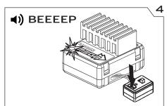
Once you have the mode you want to change selected, press and hold the setting button again. The status LED of the ESC will start flashing green. You are now in adjustment selection.
