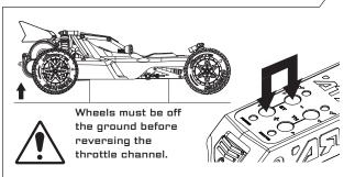
If the steering direction is reversed - i.e left goes right, check that the transmitter and receiver are switched on then simply hold both the steering trim buttons on the top panel; a long beep will sound and the steering LED will light (or go out if already lit) which signifies that the channel has been reversed.
